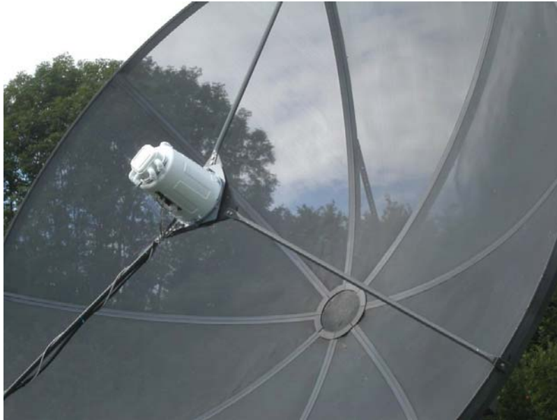
Figure 1 3m diameter dish with integrated feed / LNA
