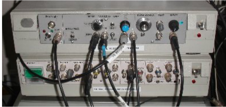
Figure 3 Post detector scaling and integration electronics
